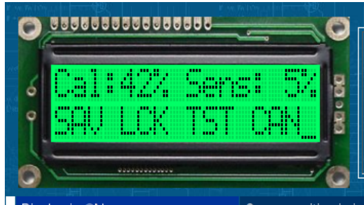
Figure 2: Design of Calibration Menu including use of “softkeys” on screen
